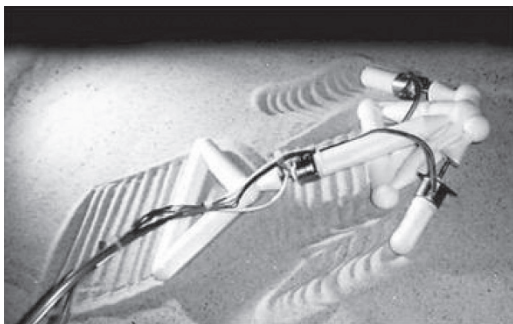
Evolutionary Robotics. Figure 7. A fully automatically evolved robot developed on the Golem project (see text for details). Used with permission
